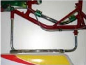
**Rear Crash Bar Adjustment:** The lower rear bar reacts similar to the rear torsion bar, however it has a much smaller affect. Tightening will increase rear grip while loosening it will help free the kart up. Since the Supersonic V uses a bearing mounted bumper, this change has no affect on this model and the bar should always be left loose.
