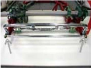
**Upper Front Bumper Bar Adjustment :** The bolts for the upper front bumper should be attached with a rubber spacer and be firmly tightened but no too tight. Loosening these bolt will reduce front steering/grip.
